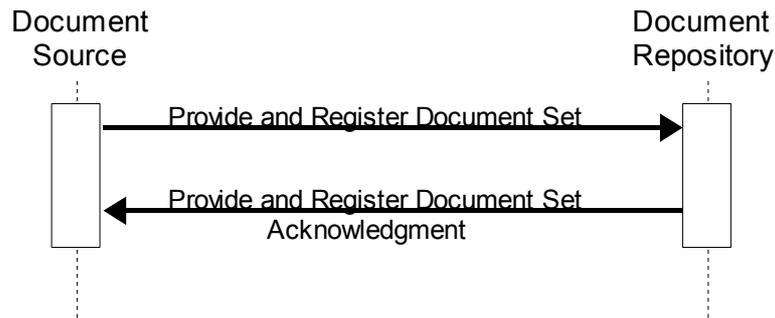
353 Figure 4: "IHE Provide/Register Document Set" Transaction Sequence Diagram
